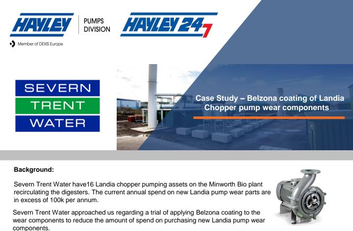
Severn Trent free issued new Landia wear components consisting of Front wear plate, Back wear plate and Volute casing, Grit blasted new components to achieve correct surface profile in line with SA2.5 Applied Belzona 1321 Abrasive Resistant coating.
